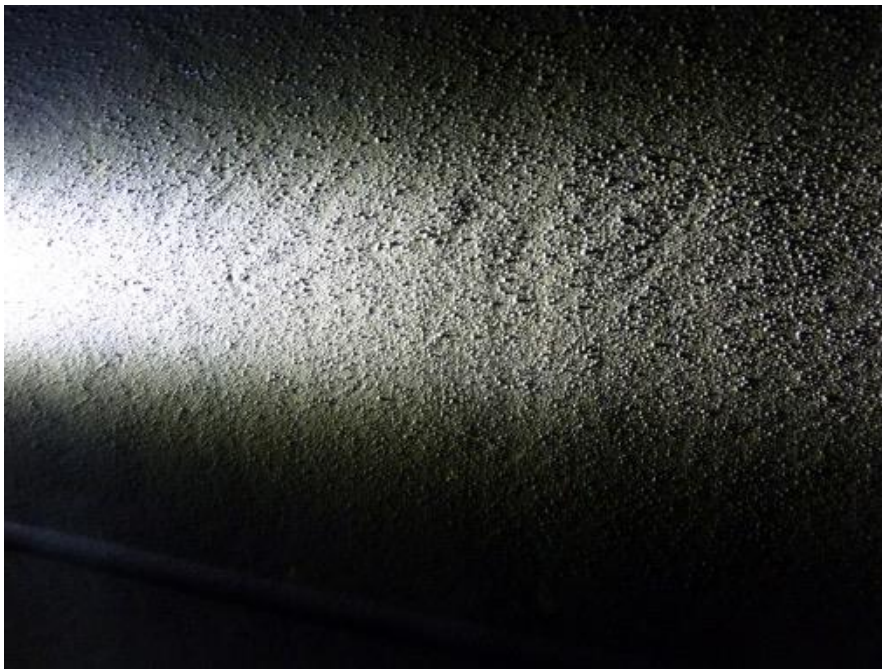
Figure 25: Cleaning level 4.3.x.x Blisters in the rubber lining
