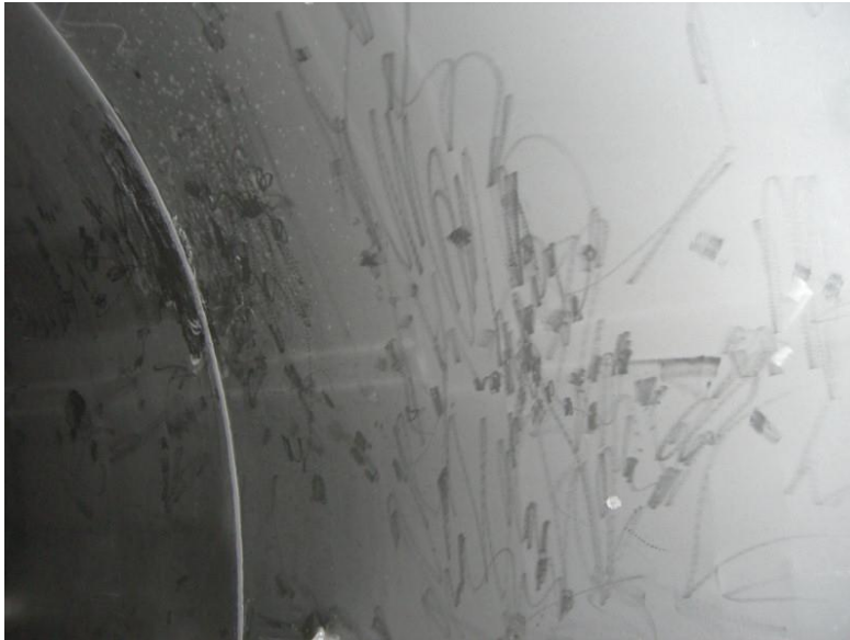
Figure 16: Cleaning level 3.2.x.x Grinding marks
