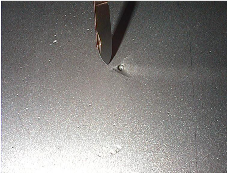
Figure 22: Cleaning level 3.6.x.x Pitting in the wall
